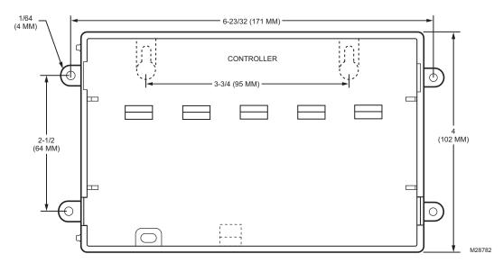
Fig. 2. Controller mounting tab dimensions in inches (mm).
